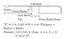
Then allow 0.5 to 1mm for additional clearance which would give a suggested dimension at "X" of 10.5mm.
